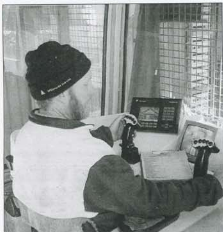
• New computer controls have been installed at the Bright Street Mill to enable log scanning, better positioning and the selection of the most effective cutting patterns.
